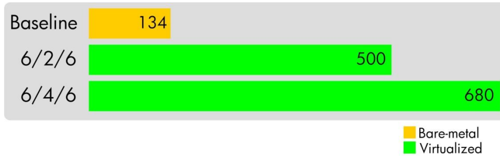
Figure 2. Showing the performance impact of enabling Intel HT Technology in a XenApp server 7
