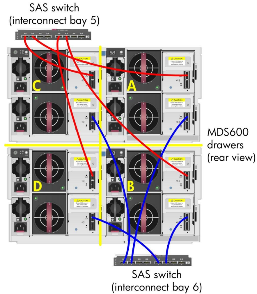
Figure A-2. SAS cabling, as pre-configured by HP
